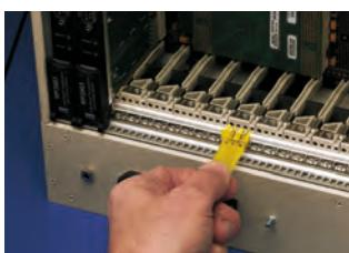
For simple assembly of keys. Up to 3 coding keys may be fitted simultaneously. An integral alignment pin makes positioning easier.
