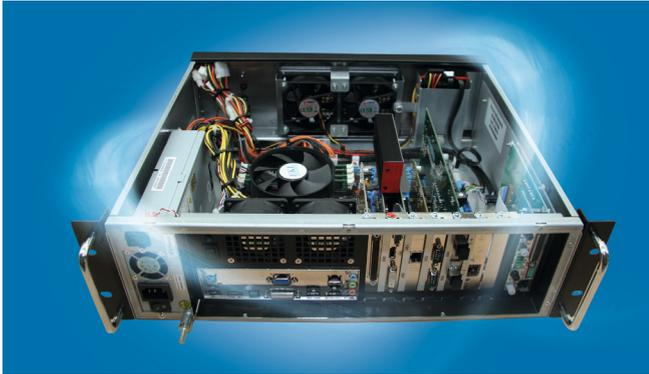
A chassis designed and manufactured by HEITEC for use as sub-assembly test equipment, including application-specific electronics
